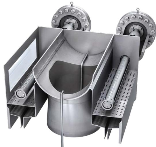
Alfa Laval's unique Spray Bar technology ensures effective mixing of the liquid feed and the recycle gas. The gas enters from the bottom and passes the Spray Bars where the liquid feed is sprayed into the gas.
