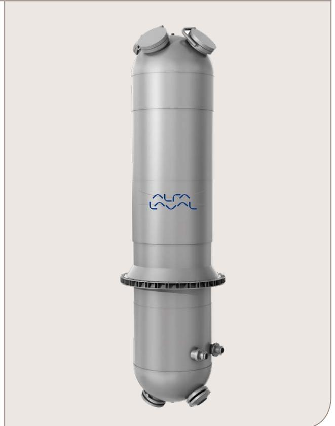
The plate bundle resides inside a pressure vessel filled with the cold-stream gas under high pressure. This means the plate bundle is only exposed to the differential pressure between the hot and cold streams, thereby minimizing the mechanical stress on the plate welds.
