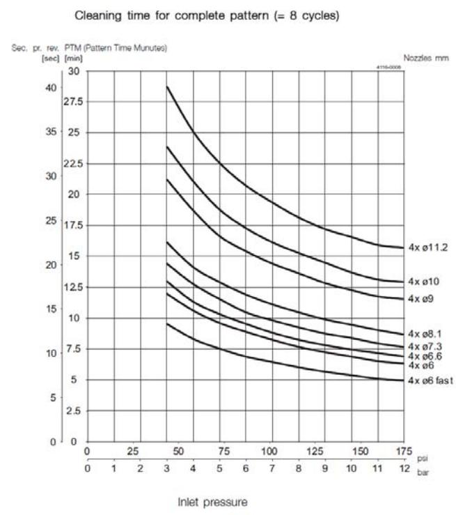
Burst cleaning version has a 20-25% faster complete pattern
