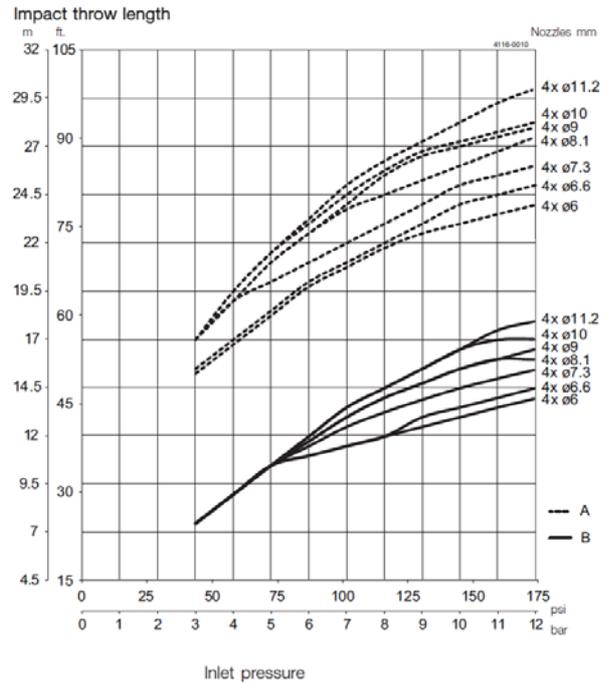
Throw length measured according to tech. specification 93P003
